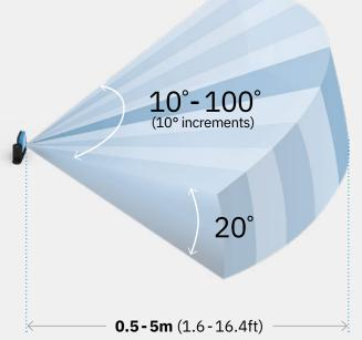
The aperture of each field is dynamically adjustable in 10° increments over a range of 10° to 100°.
