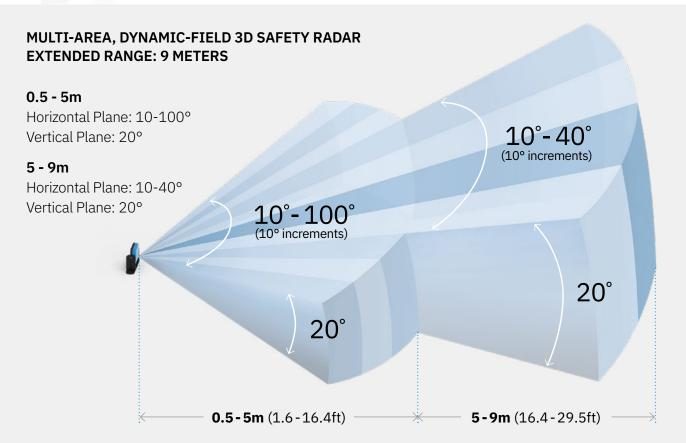
The aperture of each field is dynamically adjustable in 10° increments over a range of 10° to 100° (between 0.5 and 5 m) and over a range of 10° to 40° (between 5 and 9 m).
